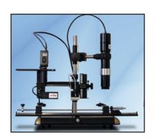
Another development from PDR is our high resolution CCTV/split beam prism-based BGA alignment option, which allows the operator to view the PCB and component simultaneously with a colour video monitor and zoom lens.
