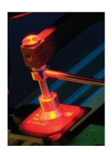
PDR's process involves pre-heating the PCB from below with a back heater and then heating the component from above. This reduces the time and energy required for topside heating, thereby minimising the potential for damage to the component, the PCB or adjacent devices. PDR's closedloop temperature monitoring system, with a non-contact IR sensor, makes the process highly controllable and repeatable, producing high quality solder joints every time.
