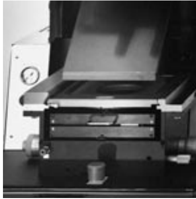
Quick conversion from mask aligner to bond aligner
