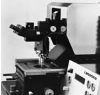
Alignment and exposure with SUSS MicroTec MA6 Mask Aligner
