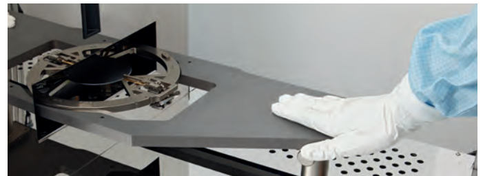
Material handling unit for ergonomic and contamination-free wafer loading
